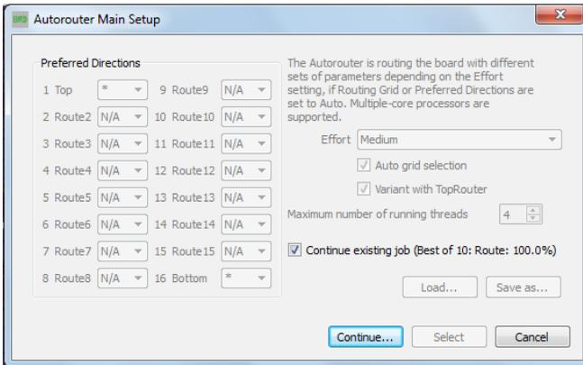
► *Autorouter Main Setup: Restarting an interrupted job*
