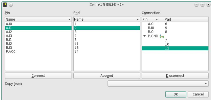
➤ **Connect: One pin is connected to three pads in Any mode**
