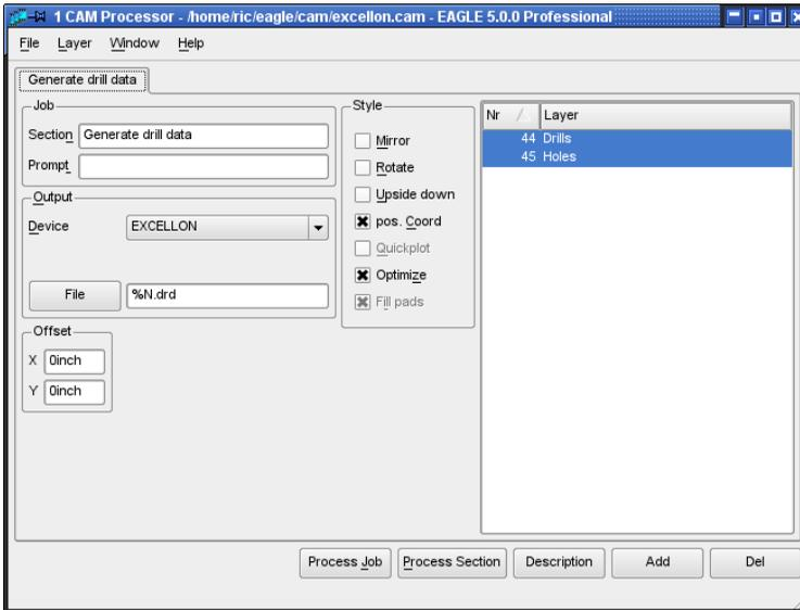
➤ **CAM Processor: Generate drill data with the excellon.cam job**
