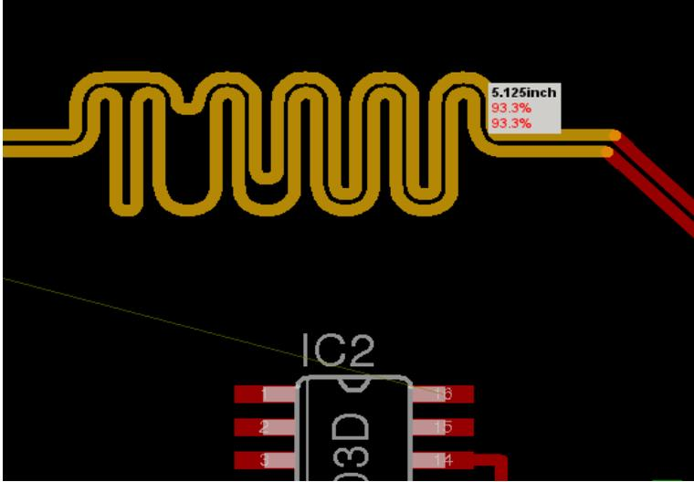
➤ **Length Display:** Target length 5.125 inch, currently both signals reached 93.3%
