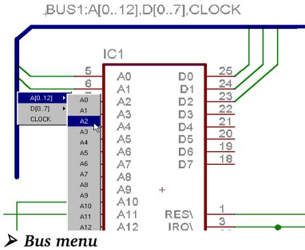
The index of a partial bus name may run from 0 to 511.
