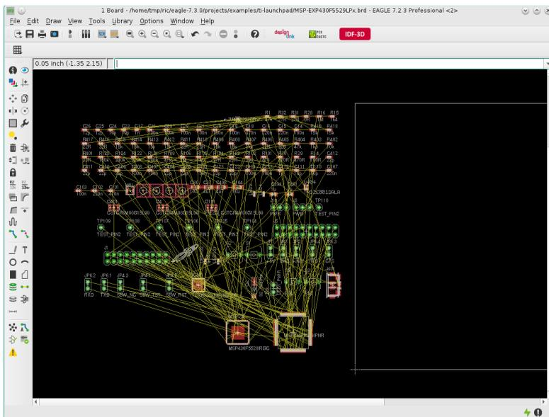
➤ **Board command:** *Create the layout from the schematic*
