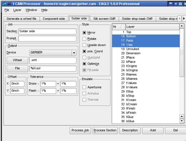
► CAM Processor: Solder side section of the gerber.cam job
