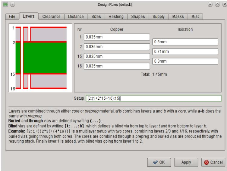
➤ **Example 2: Layer Setup for a 4 layer Board**
