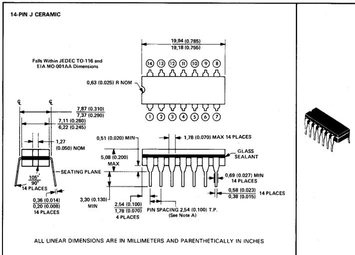
NOTE A: Each pin centerline is located within 0,25 (0.010) of its true longitudinal position.
